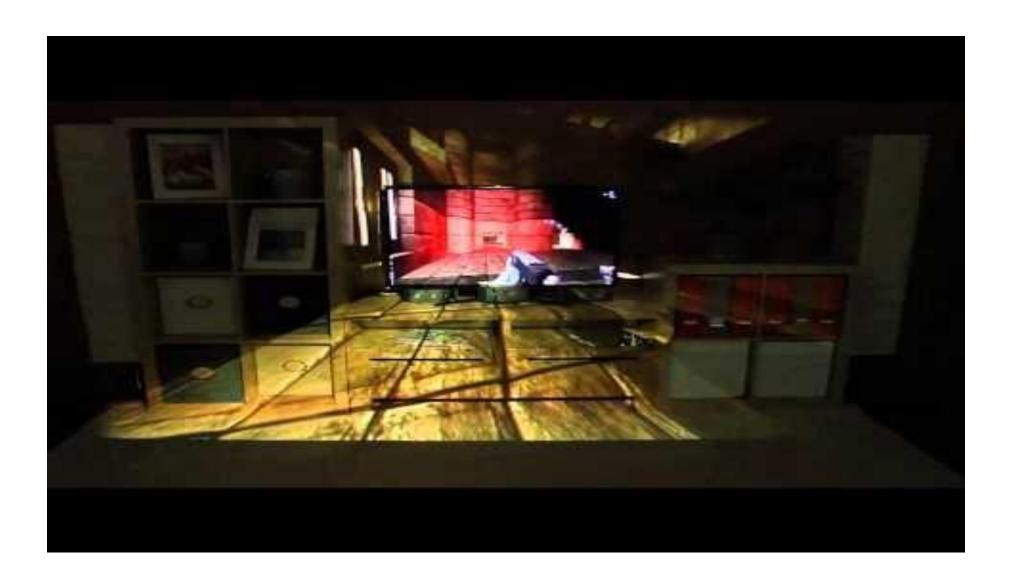
• Each projector projects a series of Gray code patterns in turn. These are captured and saved by all Kinect color cameras. Gray code patterns are used to map from a given pixel coordinate in the Kinect color image to a pixel coordinate in the projector. All cameras observe the Gray code patterns in order to establish which cameras belong to a given 'projector group' (see above). Additionally, the depth image from each Kinect depth camera is saved.
